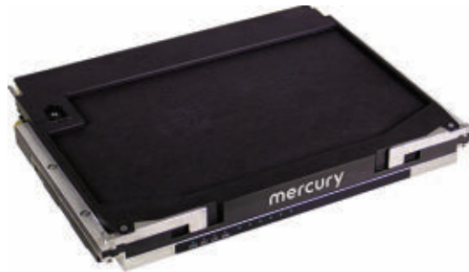
The Mercury new 6U OpenVPX use the latest Intel Xeon D-1700 processors, which were formally code named Ice Lake D.
